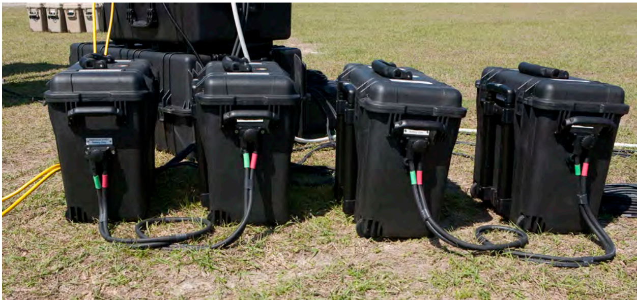
Figure 10 -Expander Paks connected using 5' Inter-connect cables
