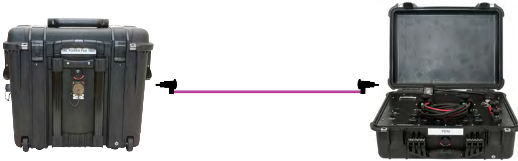
Figure 9 -Connecting PDM to Mil-Series Power Pak “LOAD” port
