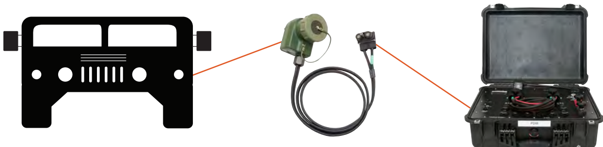
Figure 10 -NATO 24VDC to PDM
