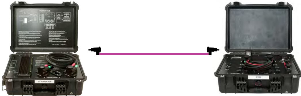
Figure 8 -Connecting PDM to Power Hub “LOAD” port
