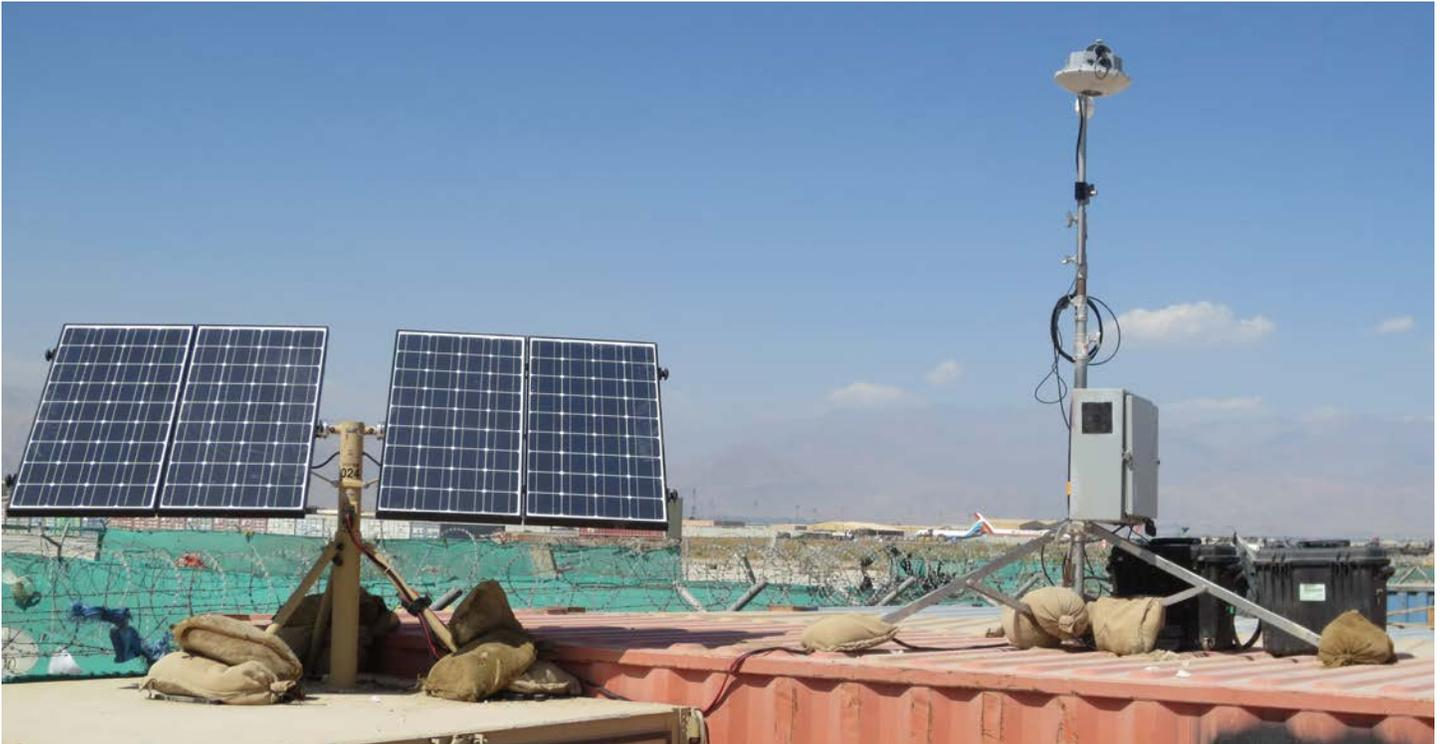
Figure 1 - RFID Interrogator System with Solar Stik Power Solution
