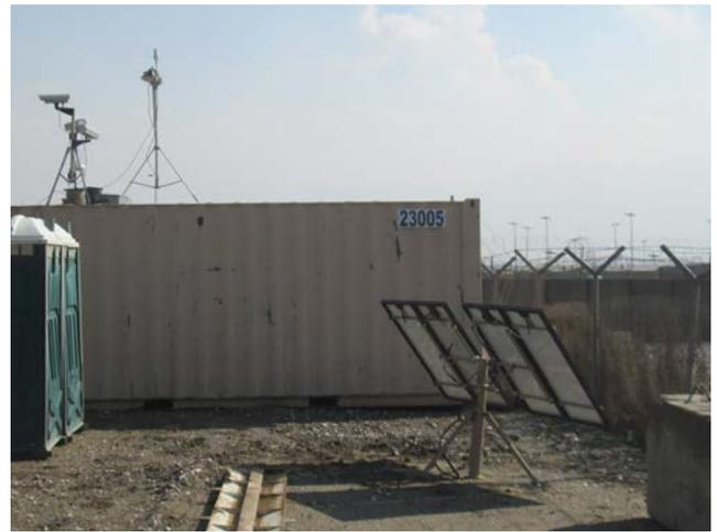
Figure 2 - Solar Stik System powering RFID Interrogator in an Afghani truck yard
