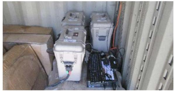
Figure 4 - Solar Stik Solution powering Interrogator System with a computer
